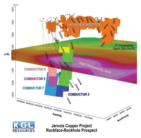
Figure 2. Rockface Prospect DHEM conductors and IP chargeability perspective view (looking southeast).
